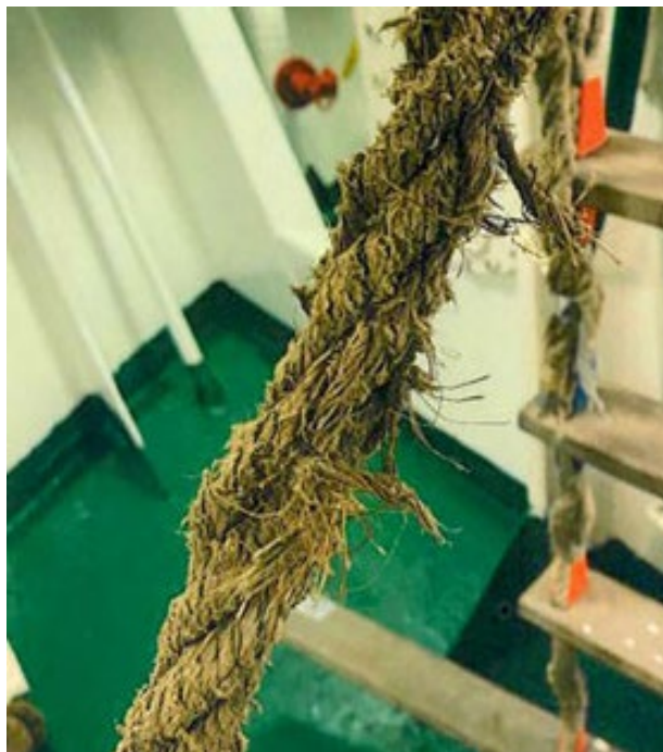
Photo 10: Frayed side rope.
