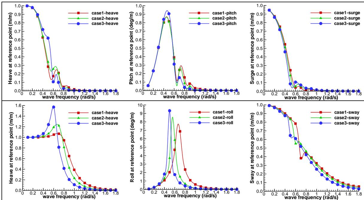
Fig. 4 Seakeeping characteristic in different loading conditions in head sea (top) and beam sea (bottom).
