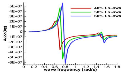
Fig. 7 The added mass in transversal direction
