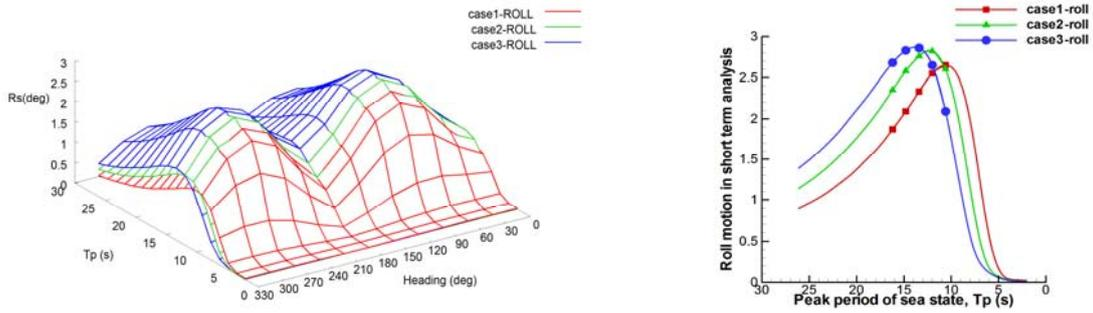
Fig. 5 Significant responses of roll motions in different wave incident angles (left); Roll motions take from left figure in 90 degree heading (right).
