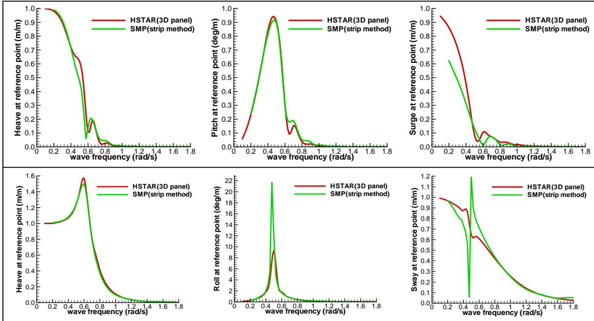
Fig. 3 Comparisons of HydroSTAR and SMP in head sea (top) and beam sea (bottom).
