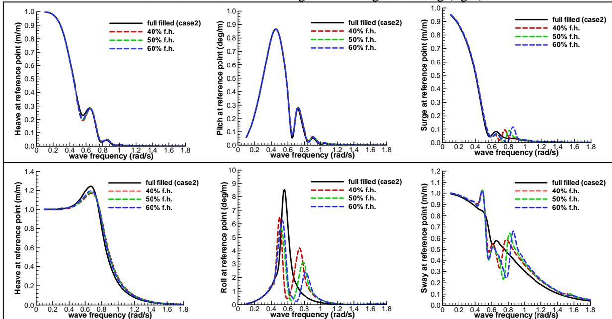
Fig. 6 Seakeeping characteristic for different filling heights tank in head sea (top) and beam sea (bottom).
