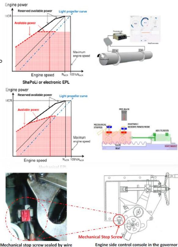
Mechanical stop screw sealed by wire
