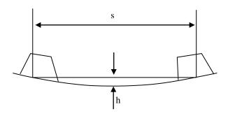
Figure C3.7.1 Measurement of Curvature
