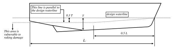
where: T = maximum draught of the hull (each hull considered individually in the case of multhulls) to the design waterline, excluding any non-buoyant structure, provided that structures such as single plate skegs or solid metal appendages shall be considered to be non-buoyant and thus excluded.
