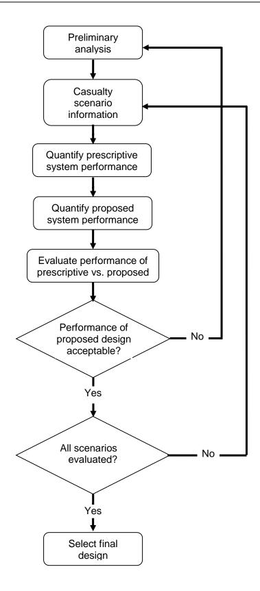
Figure 6.4.1 Alternative design and arrangements process flowchart
