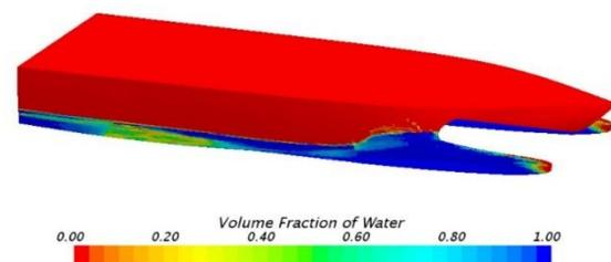
Fig. 3 Free surface representation on the ship hull.
