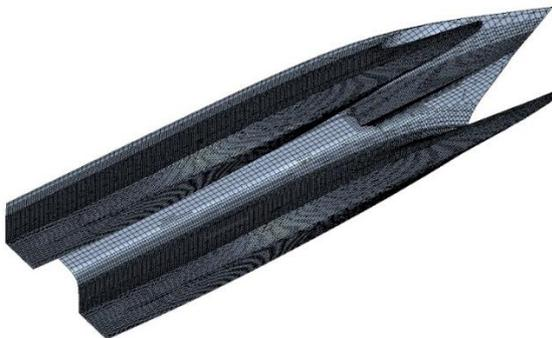
Fig. 6 Surface mesh on the hull.
