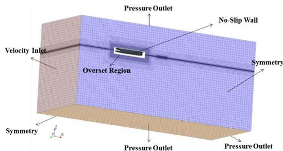
Fig. 4 A general view of the background and overset regions and the applied boundary conditions.
